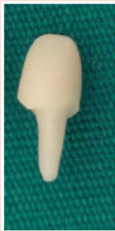
Figure 7: Zirconia post-cores after sintering.
