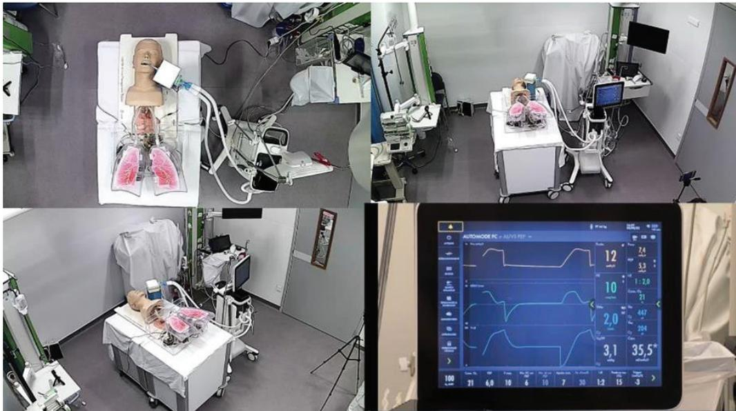
**Picture 1:** The pulmonary compliance module consists of two test balloons with elastic specificities mimicking a pulmonary alveolus.
